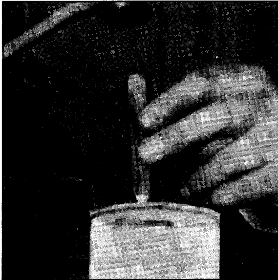
Applying Mold Marking with Stamp
